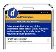
Choose a derived parameter. Options vary by installed sensors.
